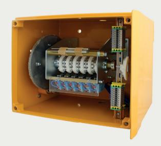
The gear limit switches with transmission ratios from 5:1 to 15:1 are modular switching devices for the pivot range limitation. The positively activated contacts are actuated by means of two infinitely variable cam discs over a zero-play toothed gear drive realized by means of a pretensioned twin gear wheel. Encoders or potentiometers can
